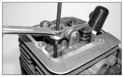
2. Loosen adjuster locknut so that the 2.5 mm Allen socket head adjustment screw can turn freely.
